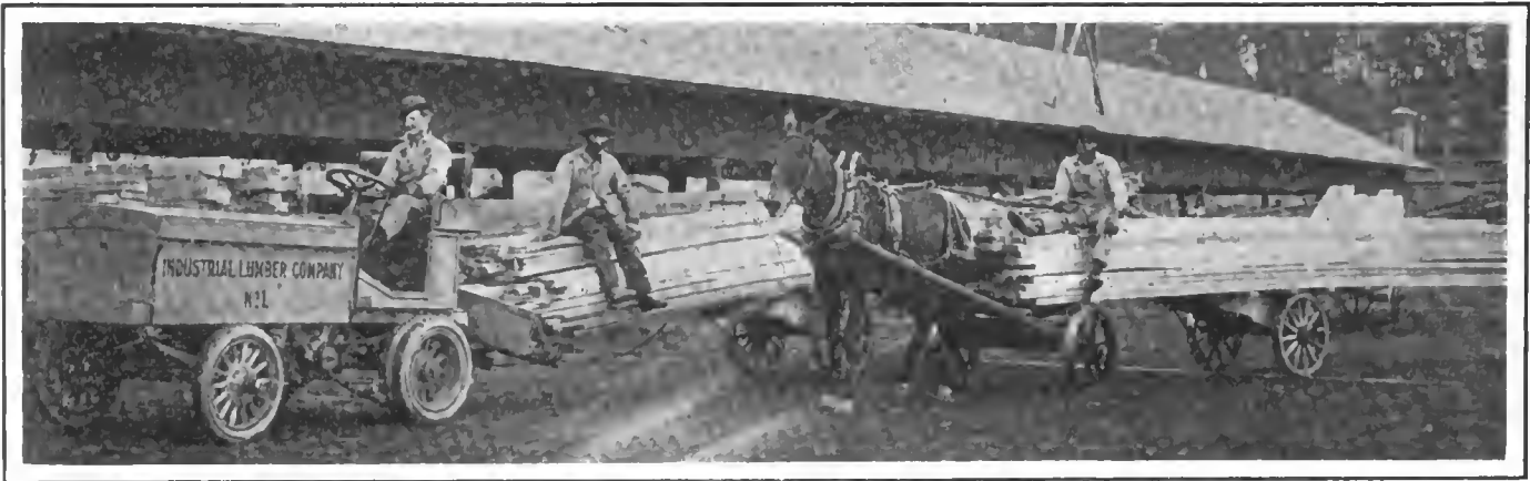
Two-ton electric lumber tractor with trailer. The batteries are situated in a single front compartment and the lumber is mounted on a two-wheeled truck. The old and new methods are contrasted
